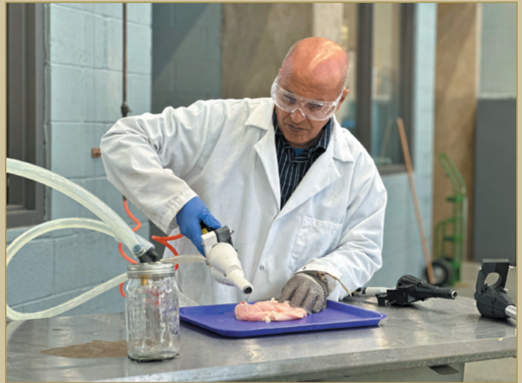
Aklilu Giorges, principal research engineer, conducts tests on butterfly chicken breast fillets using the semi-automated trimming device. The patent-pending tool is lightweight and ergonomically designed to assist poultry plant workers with removing unwanted cartilage, bone, and fat from chicken breasts while reducing excess trimming, thus increasing overall yield.
